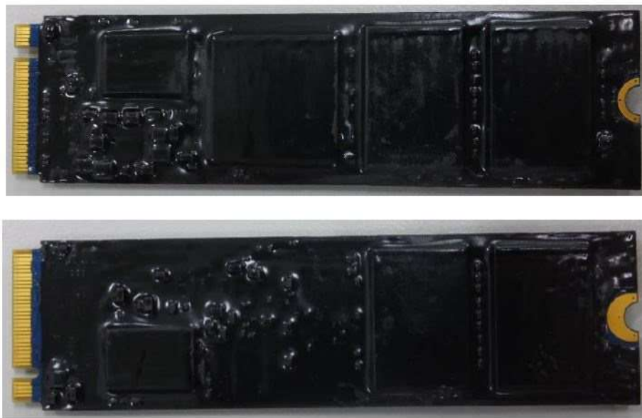
Figure 5 Example of FIPS tamper-evident epoxy resin
