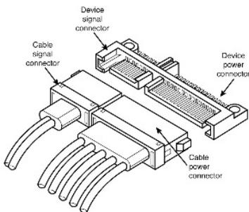
The Serial ATA interface cable consists of four conductors in two differential pairs, plus three ground connections. The cable size may be 30 to 26 AWG with a maximum length of one meter (39.37 in).
