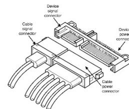
**Figure 1 Attaching SATA cabling**
