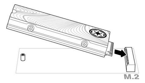
8. Hold down Beskar<sup>™</sup> Ingot Drive while you fasten the mounting screw. Make sure the SSD is secured in place.
