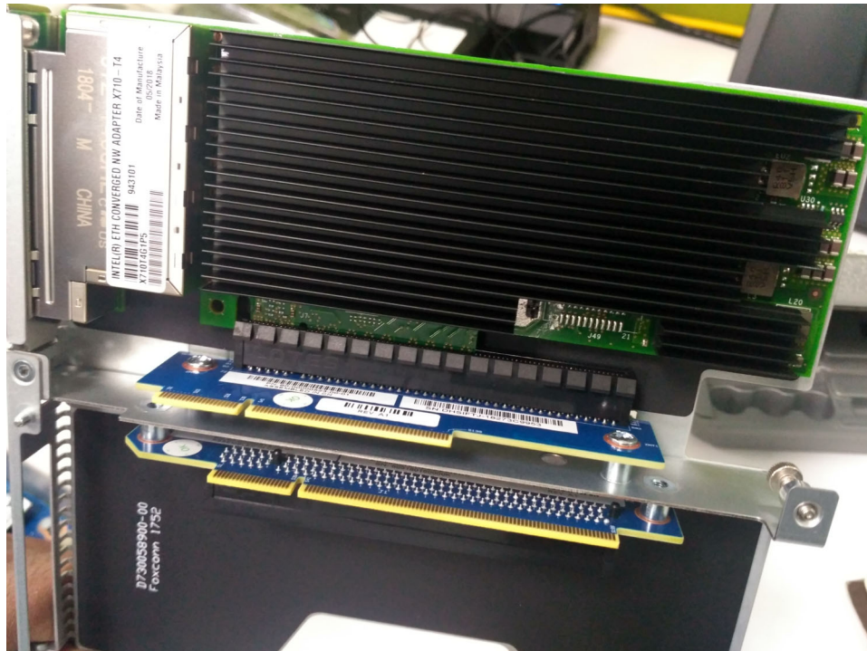
Figure 95 Inserting PCIe card (Ethernet card in this case) into the PCIe riser card
